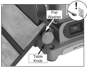
Figure 4. Installing disc table.
